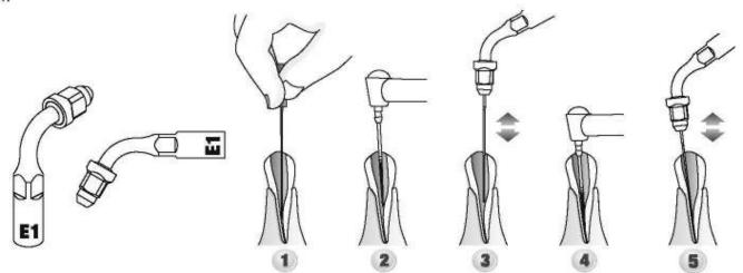
Use only the provided flat wrench to tighten the file holders on the handpiece, as well as for gently tightening the files or instruments in the holder. Do not over tighten.
